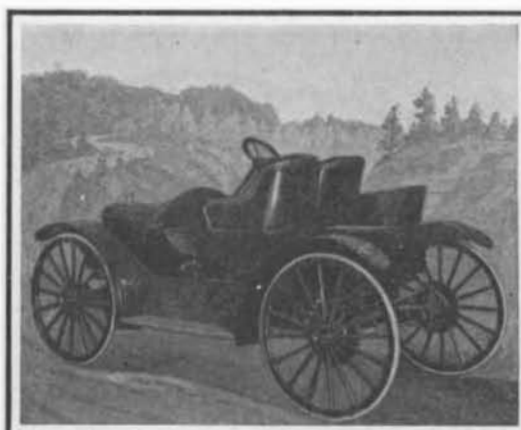
Wheel base, 95 inches; double opposed motor half offset; 16 horse-power; jump spark ignition (coil and battery).
