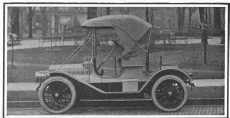
Wheel base, 95 inches; 18-20 horse-power motor; thermo-siphon cooling; mechanical oiler; jump spark ignition; friction transmission; pressed steel frame.
