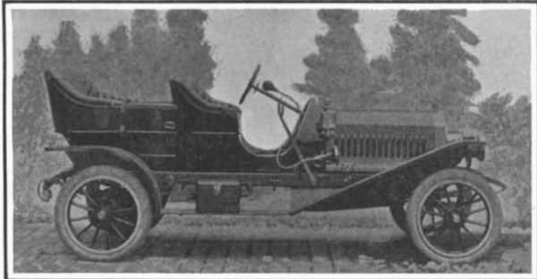
Wheel base, 110 1/2 inches; 28 horse-power; 4 cylinders, 4 x 4 inches; water cooled; jump spark ignition (storage battery); splash lubrication; single silent chain drive inclosed in dust-tight metal case; friction change gear.
