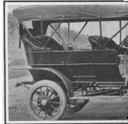
4 cylinders; 45 horse-power; speed, 3 to 50 miles unit coil; storage battery; high-tension magneto Selective sliding gear transmission. Three
