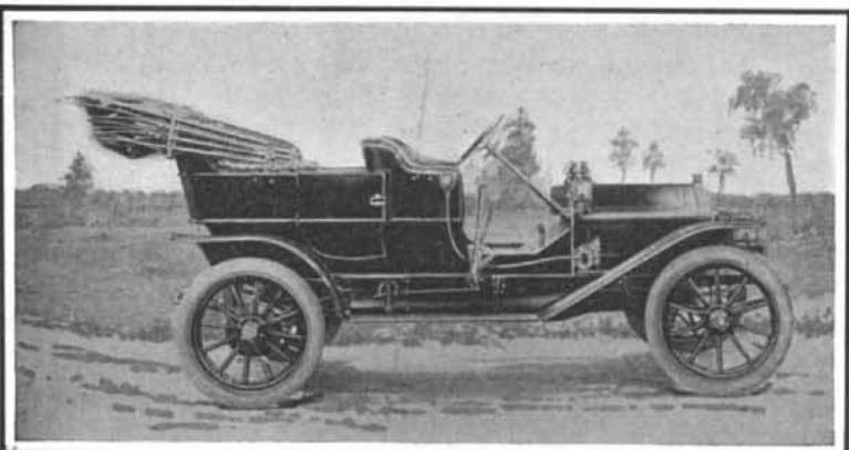
Wheel base, 106 inches; 4 cylinders, 4 x 4 1/2 inches; vertical tube radiator; dry battery and high-tension magneto ignition; expanding ring clutch; selective sliding gear transmission; three speeds forward and one reverse; shaft drive.
