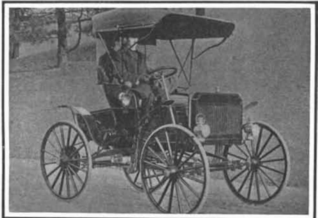
20 horse-power; 2-cylinder water-cooled motor; friction drive; force feed oiler; long Concord side springs.
