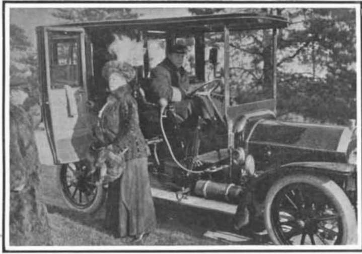
Wheel base, 117 inches; 40 horse-power; 4 cylinders, 4 3/4 x 5 1/4 inches; cellular radiator; low-tension magneto; cone clutch; selective sliding gear transmission with four speeds forward and one reverse; shaft drive.
