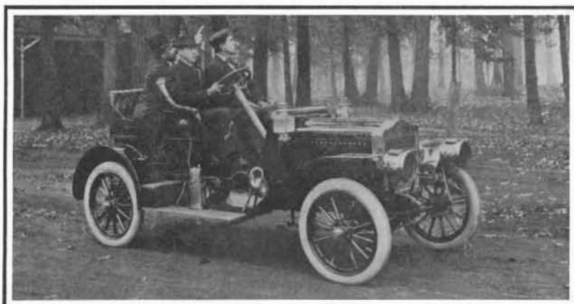
4 cylinders; 24 horse-power; magneto and battery ignition; positive shaft-driven oiler; honeycomb cooler; sliding gear transmission, three speeds forward and one reverse; bevel gear drive.
