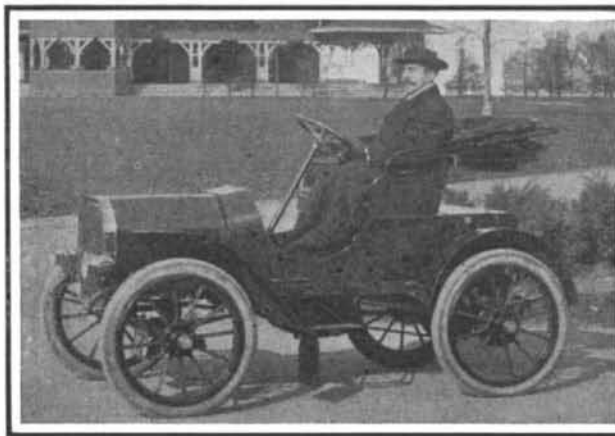
Six speeds forward, three reverse; motor, series wound, rated at 2 horse-power with 300 per cent overload capacity.
