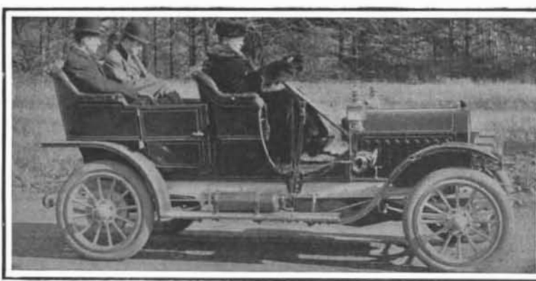
Vertical 2-cycle motor, 3 cylinders; jump spark ignition (dry and storage battery); multiple-disk clutch; shaft drive; speed, 40 miles an hour.
