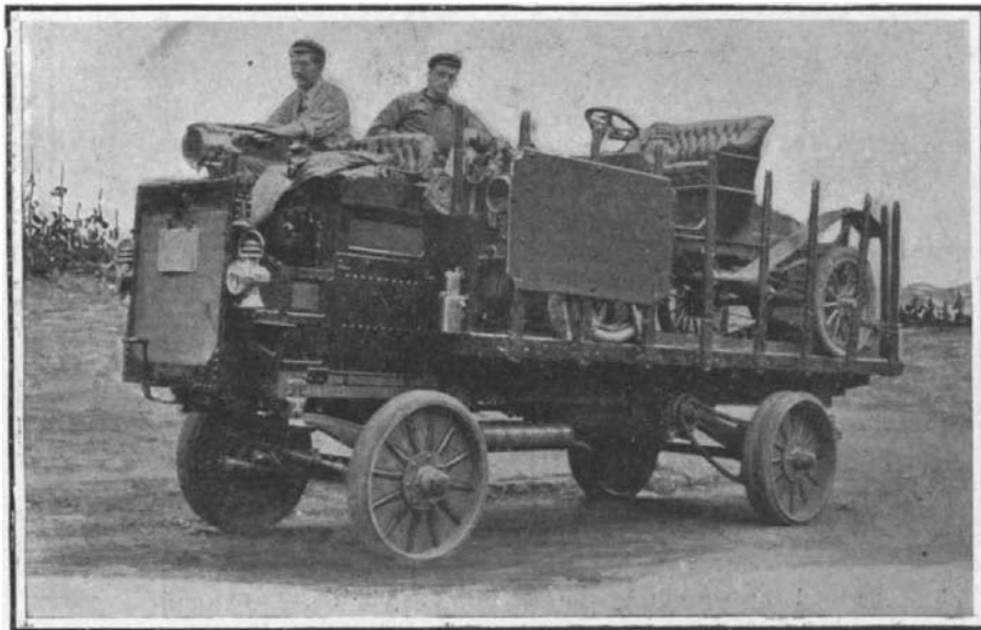
A HEAVY-SERVICE RELIANCE TRUCK. TWO-CYCLE ENGINES ARE USED.
