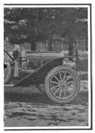
nder Rambler is a spare wheel, complete id. The regular wheel is screwed to the placed on the hub in three minutes.
