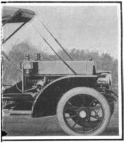
s an hour. Ignition: Jump spark; four. Irreversible bevel gear steering gear. speeds forward and one reverse.
