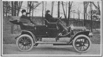
High-pressure cylinder, 21/4 x 3 inches; low-pressure cylinder, 41/4 x 3 inches. Joy valve motion actuated from connecting rods; pumps driven by levers of the valve mechanism. White steam car. 20-horse-power touring car.
