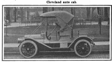
Wheel base, 95 inches; 18-20 horse-power motor; thermo-syphon cooling; mechanical oiler; jump spark ignition; friction transmission; pressed steel frame. Carter car gentlemen's roadster.
