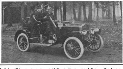
4 cylinders; 24 horse-power; magneto and battery ignition; positive shaft-driven oiler; honeycomb cooler; sliding gear transmission, three speeds forward and one reverse; bevel gear drive.
