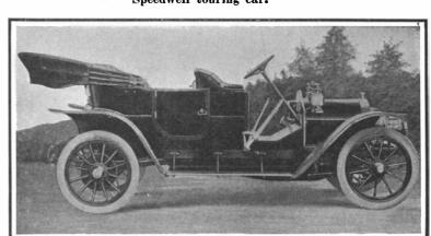
4 cylinders cast integrally; short bonnet; long wheel base; body swung between axles to give ease in riding; ignition by storage battery and coil; special equipment for double ignition (magneto with separate set of spark plugs).
