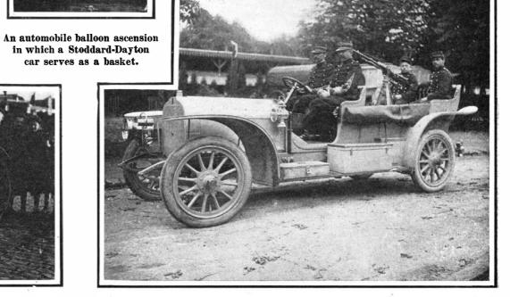
The touring car as it is used by the French army for carrying machine guns.
