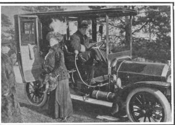
Wheel base, 117 inches; 40 horse-power; 4 cylinders, 434 x 534 inches; cellular radiator; low-tension magneto; cone clutch; selective sliding gear transmission with four speeds forward and one reverse; shaft drive.
