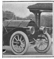
itch; selective sliding gear transmission erse; double side chain drive.
