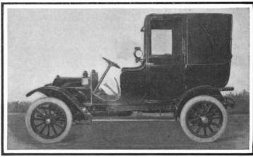
Wheel base, 106 inches; wheel tread, 54 inches; wheels, 32 x 4 inches (all four); 4 cylinders 20 horse-power; seating capacity, 4; steering on left-hand side turns in 25 feet.
