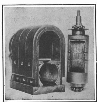
Fig. 8.—Field and armature of Bosch high-tension magneto.
