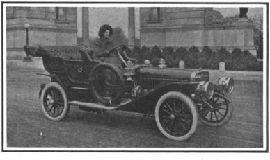
48 horse-power; 6 cylinders, vertical tube radiator; dry battery and high-tension magneto ignition; multiple-disk clutch; selective sliding gear transmission; shaft drive. Winton five-passenger car.
