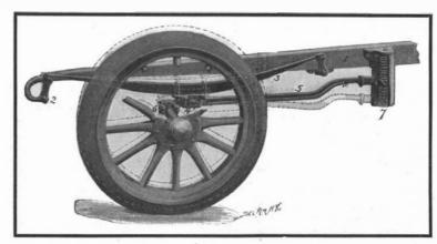
THE STOLP EQUALIZING SUSPENSION LEVER.
