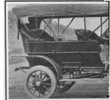
4 cylinders; 45 horse-power; speed, 3 to 50 miles unit coil; storage battery: high-tension magnets. Selective sliding gear transmission. Three
