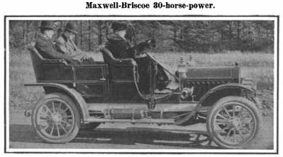
Vertical 2-cycle motor, 3 cylinders; jump spark ignition (dry and storage battery); multiple-disk clutch; shaft drive; speed, 40 miles an hour.
