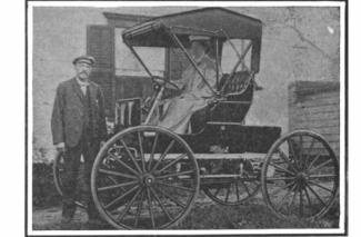
2-cylinder, 14-horse-power engine; planetary transmission; two speed forward and one reverse; maximum speed, 30 miles.
