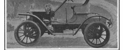
7 horse-power motor; 4 x 4 inch single cylinder; planetary transmission with multiple disk clutches. Drive: Bevel gear to jack shaft and double side chains to rear axle. Coil spring with friction joint radius rods. Maximum speed, 30 miles an hour.
