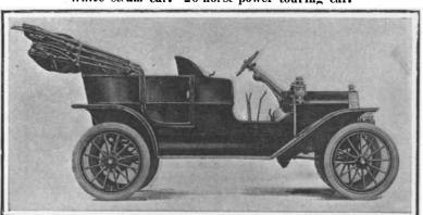
Wheel base, 100 inches; 4 cylinders; spur planetary transmission; low tension magneto ignition; vanadium steel springs, axles, shaft, gear, etc.; weight, 1,200 pounds. Ford 20 horse-power touring car.
