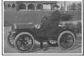
Six speeds forward, three reverse; motor, series wound, rated at 2 horse-power with 300 per cent overload capacity.
