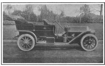
Wheel base, 120 inches: 40 to 45 horse-power; 4 cylinders 43/x 5 inches; double ignition system with Bosch magneto; cellular radiator; cone clutch; selective sliding gear with three speeds forward and one reverse; roller bearings throughout; shaft and bevel gear drive.
