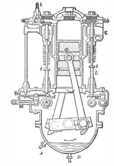
Fig. 5.—SPLASH SYSTEM OF LUBRICATION.
