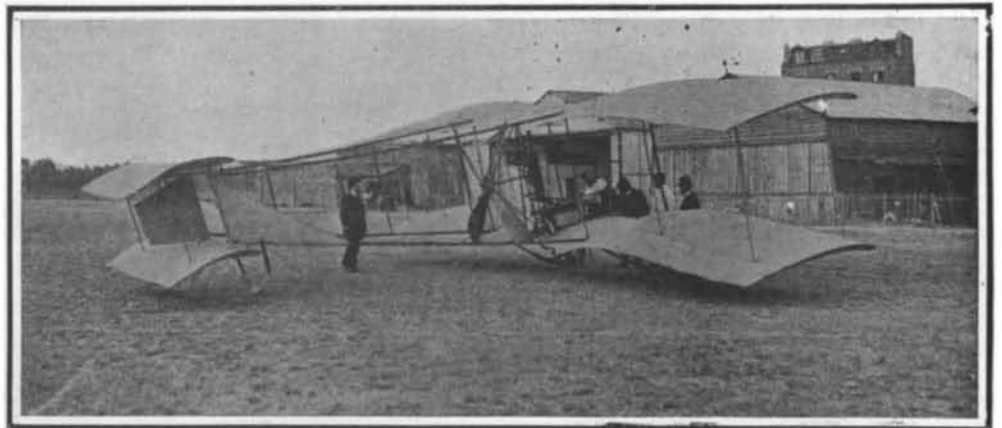
The Lepetil aeroplane—a new biplane resembling the Voisin in general outline. Note the transverse curving of the surfaces; also the four-bladed propeller.
