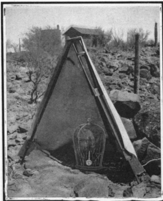
Apparatus for determining the amount of water lost from a plant by evaporation from its surface. The apparatus consists of a delicate hygrometer and thermometer, and a bell glass which covers tightly both the hygrometer and the plant. A shade is employed to avoid high temperatures in the bell. Post-like projections in background are large cacti.
