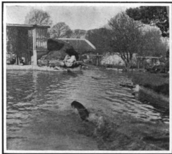
"Gyrinus" model towed backward to illustrate loss of pressure on cruiser stem and stern at high speed.
