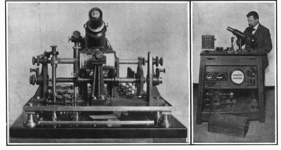
Fig. 3.—Front view of the apparatus with the cover of the cylinder removed. Fig. BELIN'S IMPROVED APPARATUS FOR THE ELECTRICAL TRANSMISSION OF PICTURES.
