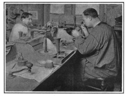
Fig. 2.-Blowpipes and oxygen cylinder in Paquier's ruby factory.
