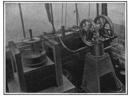
Fig. 1.-Sifting the mixture of alumina and oxide of chromium.
