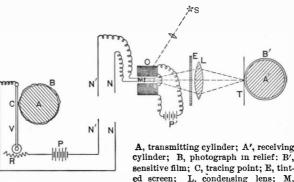
ed screen; L, condensing lens; M, mirror; NN', line wires; O, Blondel oscillograph; PP', electric batteries; R, rheostat; S, Nernst lamp; T, aperture  $_{1\overline{1}\overline{0}}$  inch diameter; V, lever-
