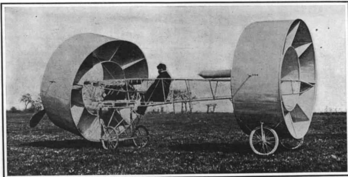
The Givaudan circular aeroplane—a new French machine of novel design.
