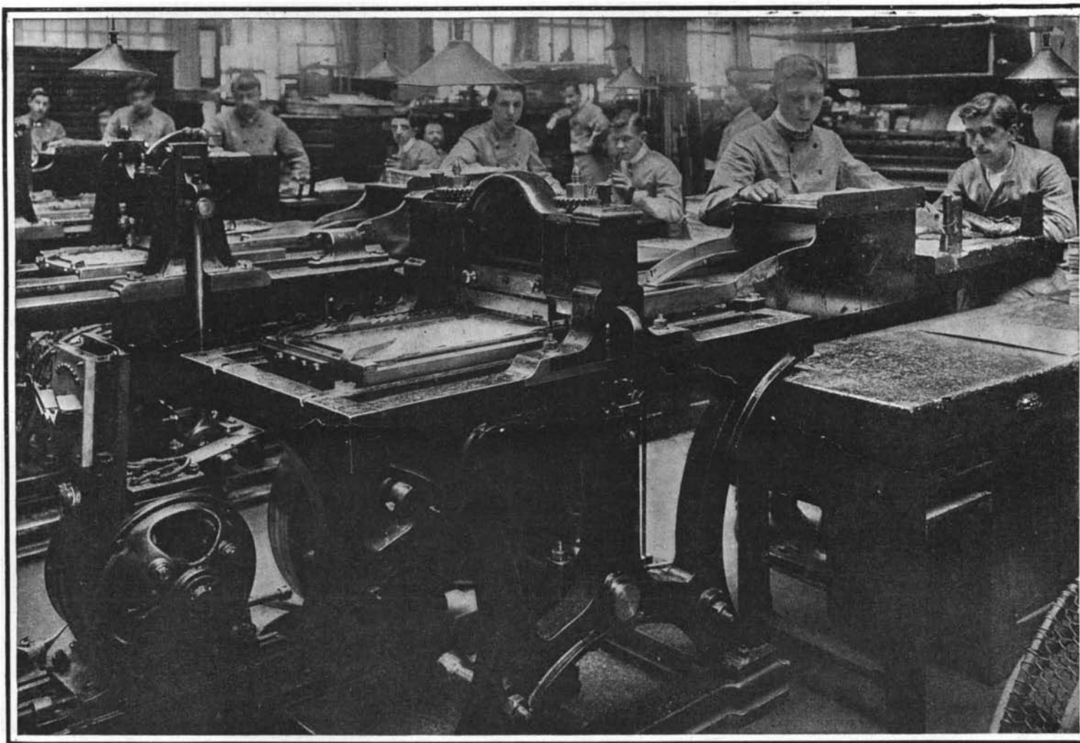
Fig. 6.—The perforating machines.
