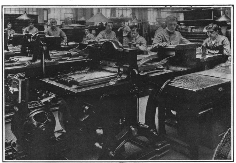
Fig. 6.—The perforating machines.
