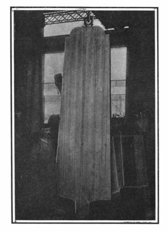
An 18-ton ingot sawn in two to show absence of piping.
