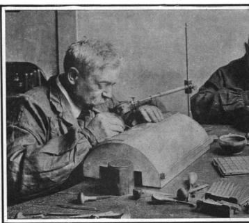
Fig. 5.—Engraving the plates from which posta;
