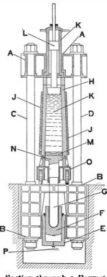
Section through a Harmet fluid-compression press.
