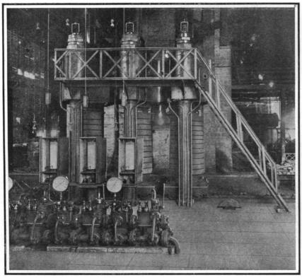
A 3,500-ton fluid-compression press capable
