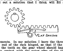
requirements. In my solution I have the three teeth on the end of the rack hinged, so that if the top of one of the teeth on the gear wheel should happen to come in contact with the outer edge of the tooth on the end of the rack, instead of jamming the teeth the hinged part will swing downward, allowing the next tooth to engage with the rack. HERBERT STARE. Malden, Mass.
