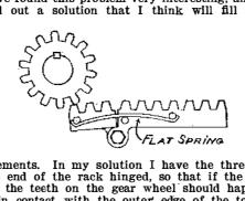
requirements. In my solution I have the three teeth on the end of the rack hinged, so that if the top of one of the teeth on the gear wheel should happen to come in contact with the outer edge of the tooth on the end of the rack, instead of jamming the teeth the hinged part will swing downward, allowing the next tooth to engage with the rack. HERBERT STARB. Malden, Mass.
