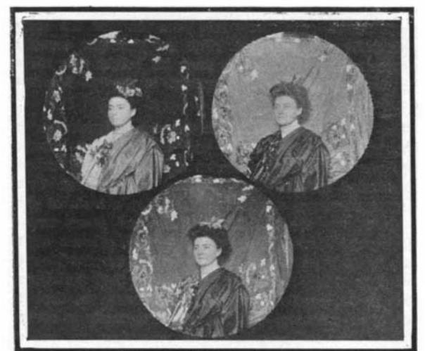
TRANSPARENCY SHOWING THE THREE IMAGES FOR PROJECTION THROUGH THE THREE COLOR SCREENS.
