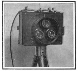
THE CAMERA WITH ITS THREE LENSES AND SOCKET IN FRONT FOR A COMMON CONDENSER.
