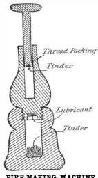
making machine which I obtained from a native in the Lobo Mountains, Batangas, P. I., and which embodies a different principle from any described in the
