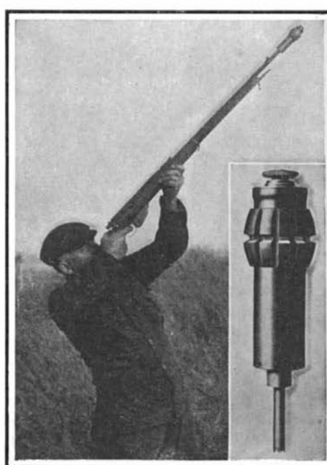
A GRENADE WHICH IS HURLED BY A RIFLE AND EXPLODED AT THE TARGET.
