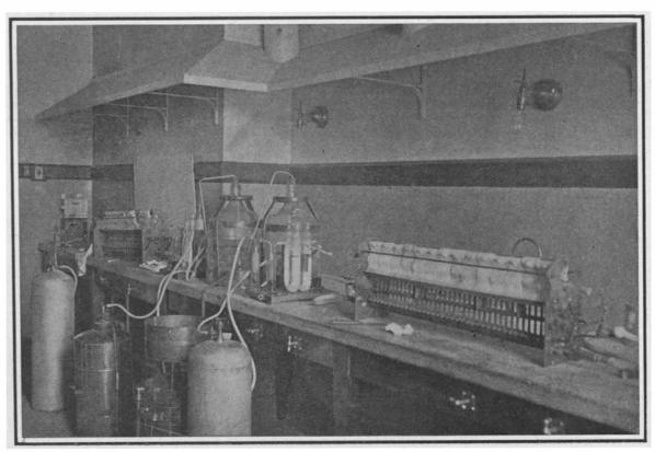
Combustion apparatus in special combustion room of the chemical department.
