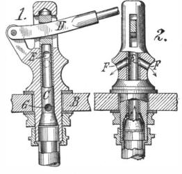
VALVE FOR FLUSH TANKS.
