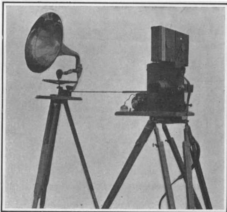
The phonograph repeats the previously recorded utterances of the actor while he performs the necessary gestures in synchronism for the moving picture machine.
