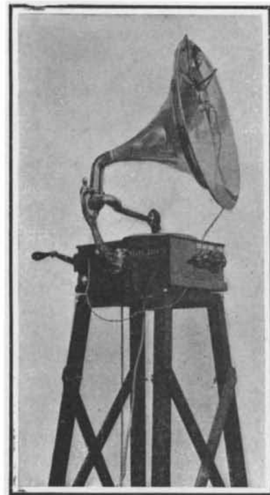
Weight-driven phonograph used to send a current into the distant moving picture machine motor.
