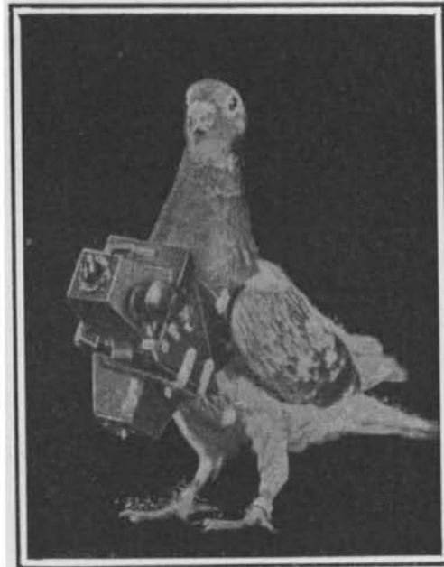
Carrier pigeon equipped with a two-lens camera.
